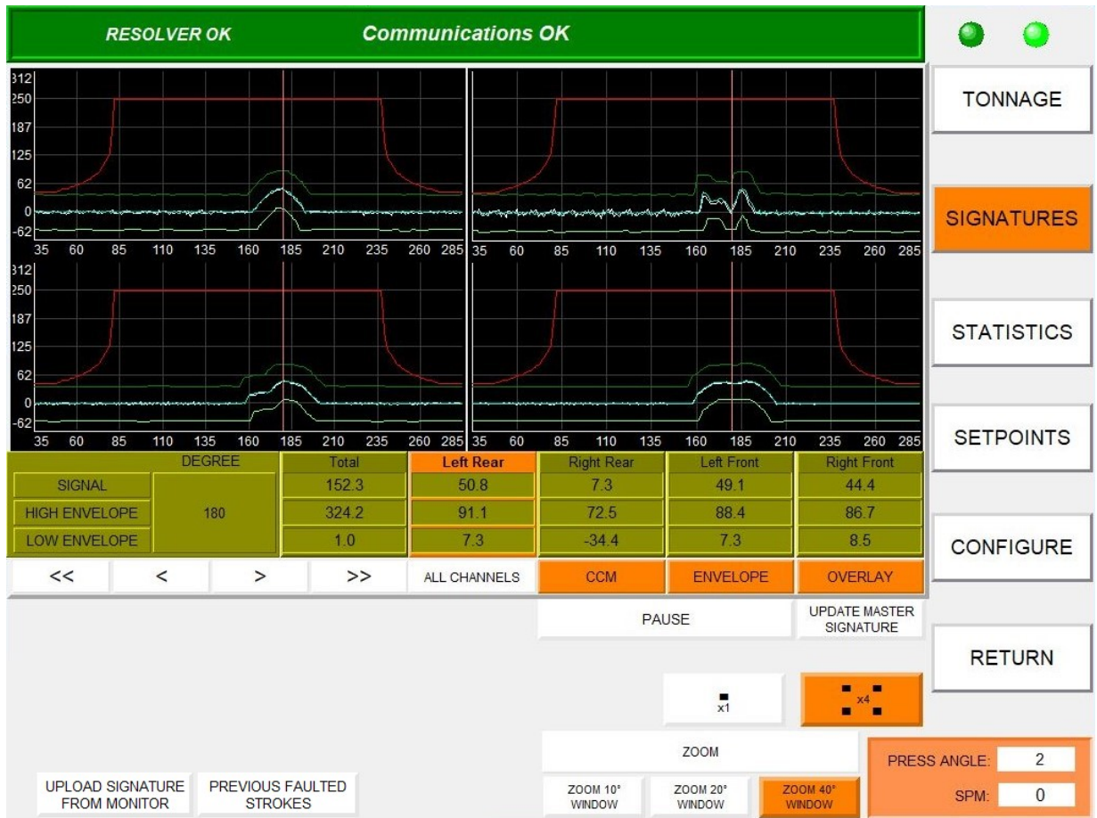
Figure 4-2 – Signature Screen (4 Channel)
