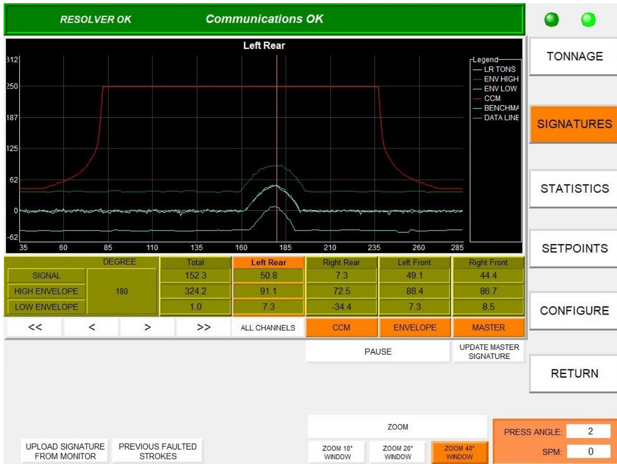
Figure 4-1 – Signature Screen (1 Channel)
