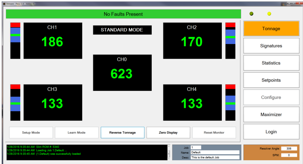
Figure 5-1 – Tonnage Screen (4 Channel)
