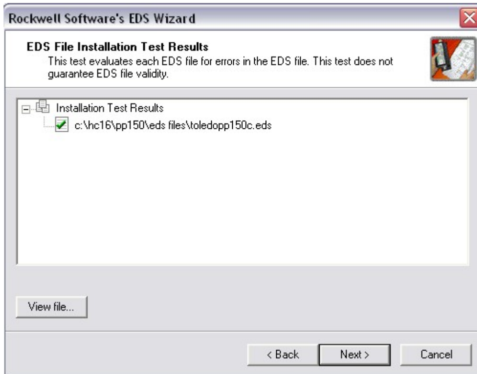
CLICK ON THE “NEXT” BUTTON TO LET ROCKWELL TEST THE FILE. (FIGURE 13.4)
