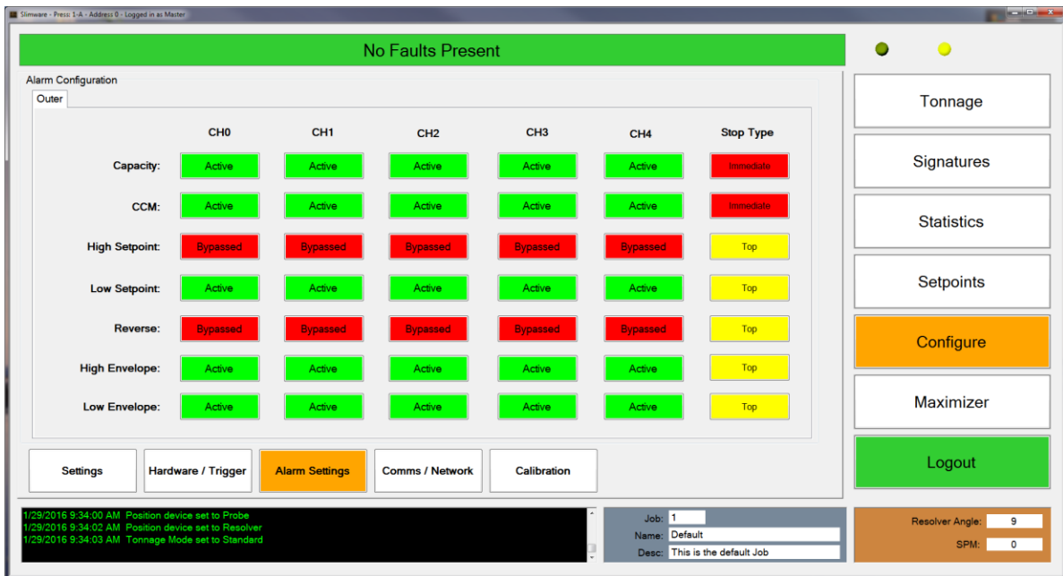
Figure 2-17: Configure Alarm Settings Screen (4-Channel)
